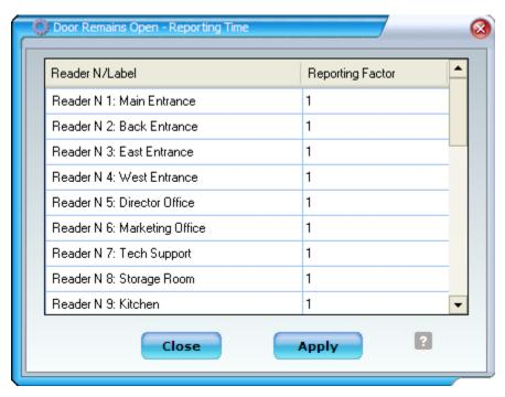
This feature allows to set the time after which the system will report that doors remains open, the reporting time valid values range from 5 seconds to 255 seconds(4.25 minutes).
